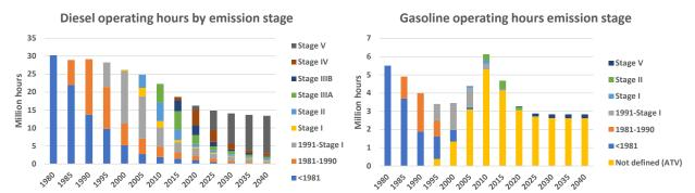
Figure 6.1.5 Operating hours by emission stage for diesel and gasoline fuelled agricultural non-road machinery 1980-2040.
