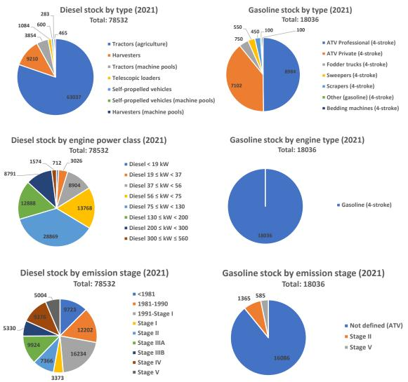
Figure 6.1.1 Stock by fuel type, machine type, engine power class and emission stage for agricultural non-road machinery in 2021.
