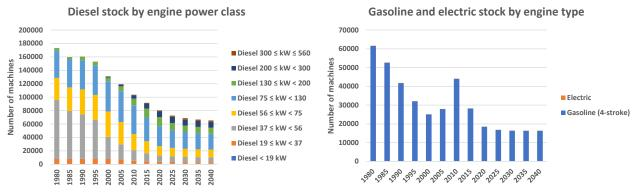
Figure 6.1.2 Stock by engine power class/engine type for agricultural non-road machinery 1980-2040.
