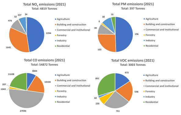
Figure S.6 Emissions of NO<sub>x</sub>, PM, CO and VOC per sub-sector for non-road machinery in 2021.
