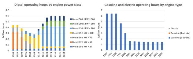
Figure 6.2.4 Operating hours by engine power class/engine type for forestry non-road machinery 1980-2040.
