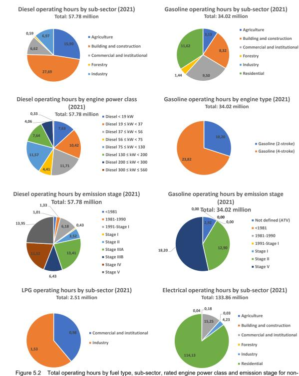
Figure 5.2 Total operating hours by fuel type, sub-sector, rated engine power class and emission stage for nonroad machinery in 2021.
