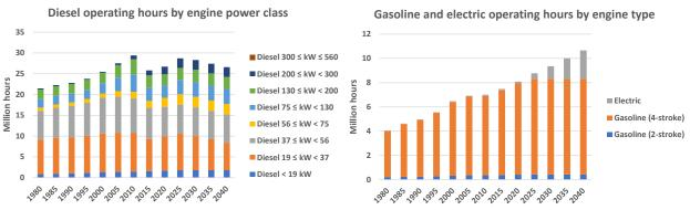
Figure 6.3.4 Operating hours by engine power class/engine type for building and construction non-road machinery 1980-2040.
