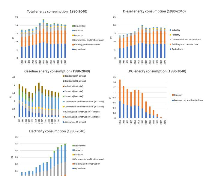
Figure S.9 Energy consumption by fuel type and sub-sector for non-road machinery 1980-2040.
