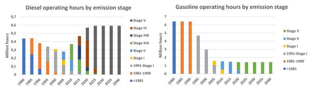
Figure 6.2.5 Operating hours by emission stage for diesel and gasoline fuelled forestry non-road machinery 1980-2040.
