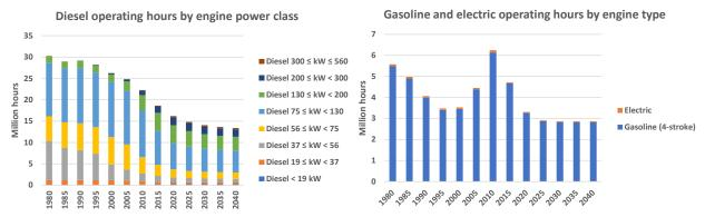
Figure 6.1.4 Operating hours by engine power class/engine type for agricultural non-road machinery 1980-2040.
