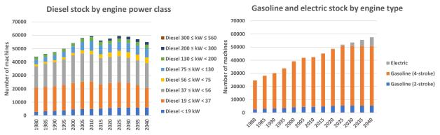
Figure 6.3.2 Stock by engine power class/engine type for building and construction non-road machinery 1980-2040.
