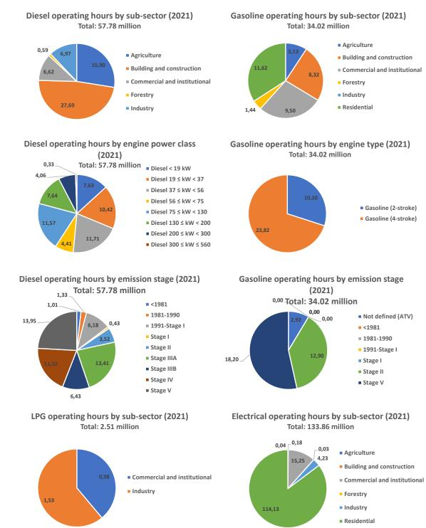
Figure S.2 Total operating hours by fuel type, sub-sector, rated engine power class and emission stage for non-road machinery in 2021.
