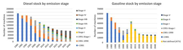
Figure 6.1.3 Stock by emission stage for diesel and gasoline fuelled agricultural non-road machinery 1980-2040.
