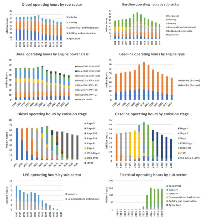
Figure S.4 Total operating hours by fuel type, sub-sector, rated engine power class and emission stage for non-road machinery 1980-2040.
