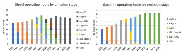
Figure 6.3.5 Operating hours by emission stage for diesel and gasoline fuelled building and construction non-road machinery 1980-2040.
