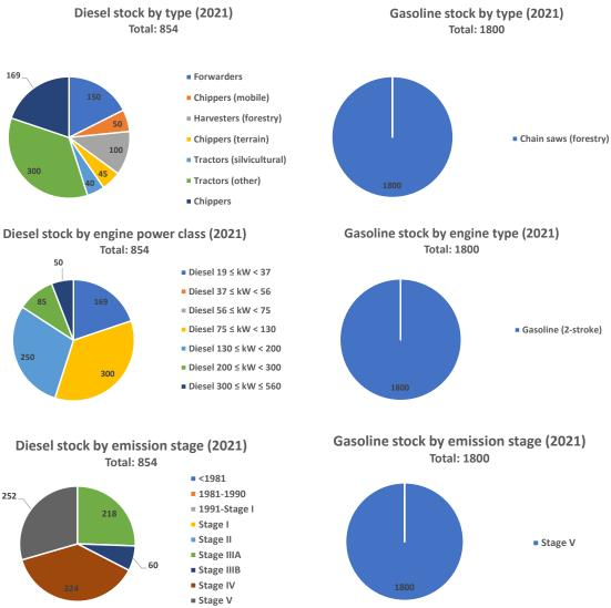
Figure 6.2.1 Stock by fuel type, machine type, engine power class and emission stage for forestry non-road machinery in 2021.
