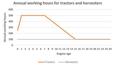
Figure 2.1.1 Annual working hours for tractors and harvesters as a function of engine age.
