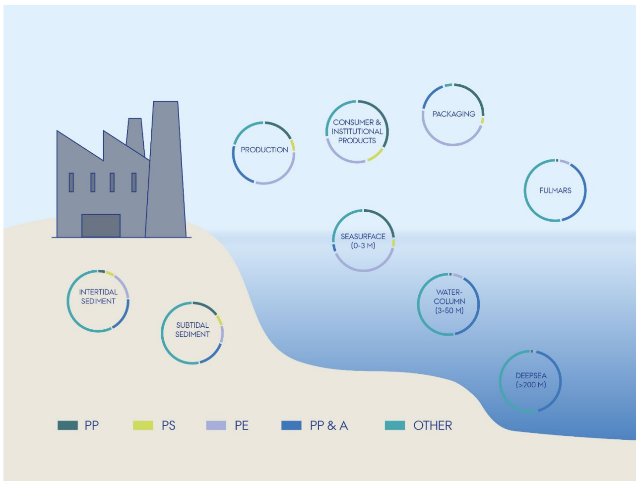
Figure 12: Composition of plastics at different stages in the plastic value chain and in the marine environment. Based on Geyer et al. (2017), Erni-Cassola et al. (2019) and Ask et al. (2020)
